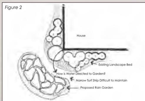
Figure 2 illustrates what often happens when a rain garden is installed but not integrated with the existing landscaping. Consider how to convey water from the landscape bed (above) to the rain garden (below).
