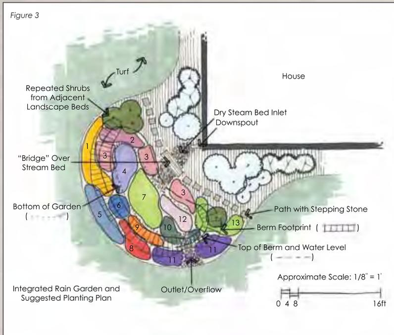
Figure 3 shows how a landscape near a house can be integrated with a proposed rain garden design. A garden that borrows or shares plants from existing or proposed landscape beds in the yard, or is physically joined with existing or proposed landscape beds, has a much stronger visual connection to the surrounding landscape. Access and maintenance can also be enhanced with beds that are linked together.
