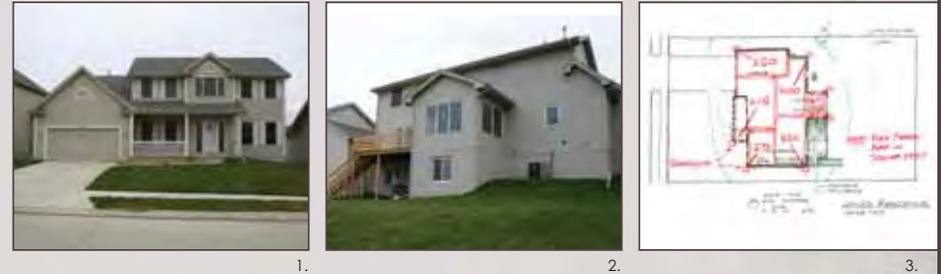
A house with multiple dormers and rooflines can be a challenge for calculating runoff. Volumes from each portion of the roof are important to separate by downspout for accurate runoff sizing. (1. Front view. 2. Back view. 3. Diagram showing roof areas.)
