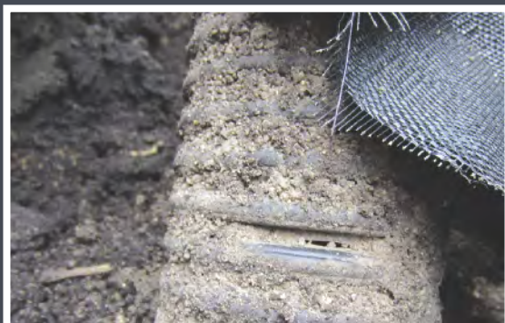
Dirty road gravel with slotted corrugated drainage pipe that clogged rapidly
