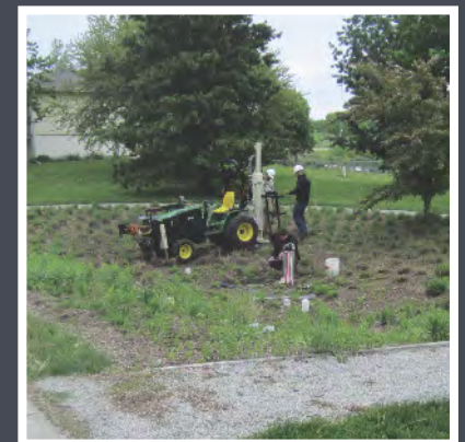
Soil cores are being taken at the Orchard Park bioretention garden to better understand plant rooting and soils.
