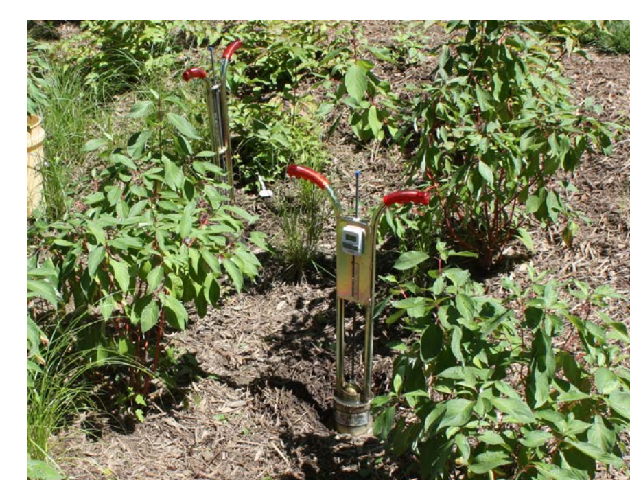
Site 10 rain garden showing infiltration tests using double-ringed infiltrometers
